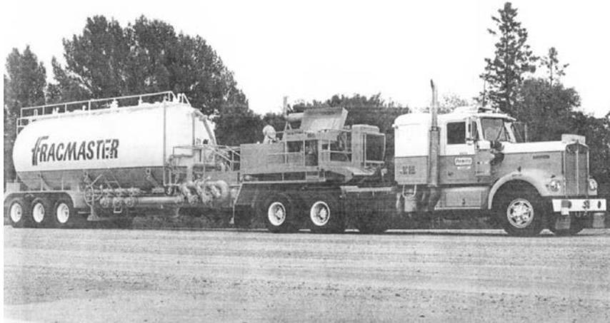
Figure 3. Liquid CO<sub>2</sub> from the truck and the solid proppant are mixed in a closed vessel and used for subsequent fracturing in the Dry-Frac stimulation. Source: Mazza, 2001
