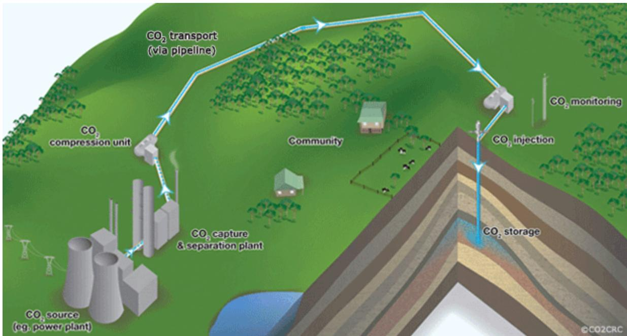
**Figure 1. CCS prevents CO<sub>2</sub> emissions from entering the atmosphere and instead stores the CO<sub>2</sub> deep underground.** Source: Global CCS Institute
