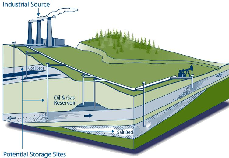
Emissions are captured from an industrial source, transported to a storage site and injected deep below ground into coal and salt beds and oil and gas reservoirs, as shown here.
