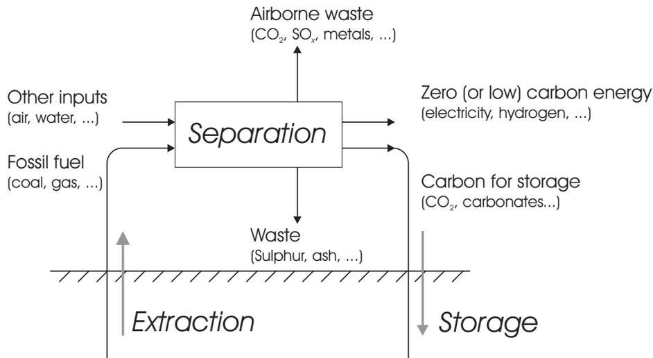
**Figure 1.** CO<sub>2</sub> capture and storage viewed as a general process for using fossil fuels with minimal atmospheric emissions of CO<sub>2</sub>.
