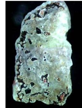
Calcite deposition on basalt (Source: PPNL)
